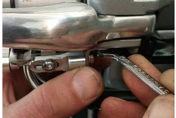
Ref. 2.D Push back on the end bracket to keep it from rotating as you tighten the brake pivot nut.
