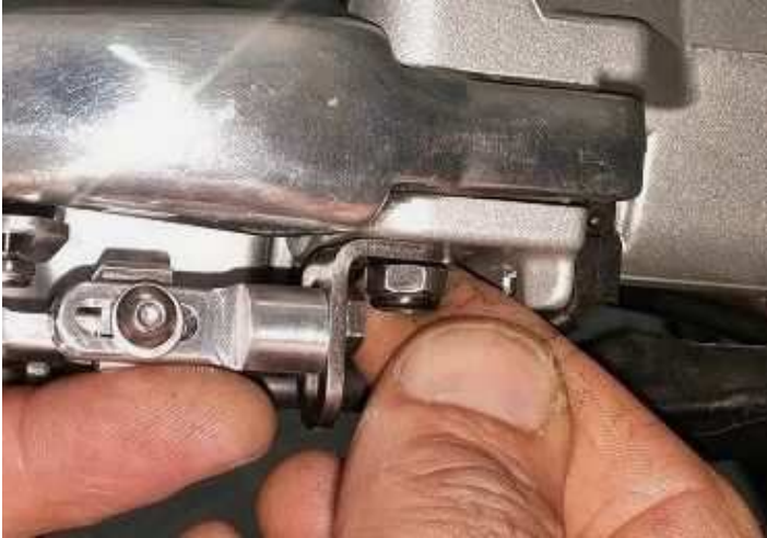
Ref. 2.C Replace brake pivot nut.
